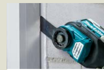
Cutting window putty, silicone
